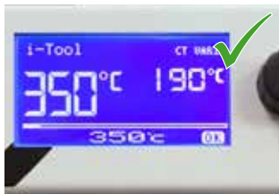
340 – 360 °C for lead-free solder
